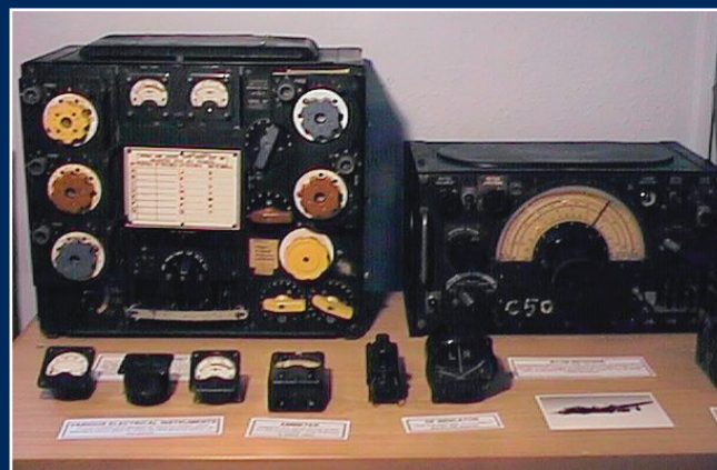
T1154 & R1155 were the transmitter and receiver used in most heavy aircraft such as the Lancaster
